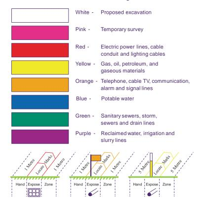
Electronic line locating is not precise and cables can deviate from their marked position. For this reason, the excavator must first fully expose the facilities by hand before using any mechanical excavation equipment within the hand expose zone. If buried facilities are not found within the hand expose zone, the locate service provider noted on the ticket should be contacted immediately so they can revisit the site and verify their markings.
